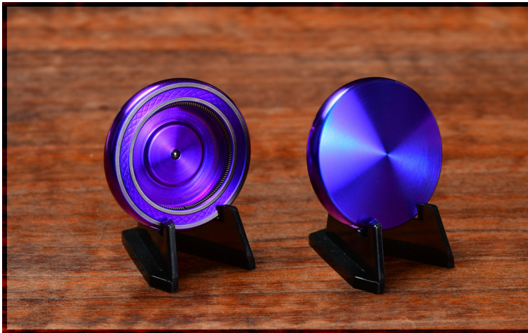
Titanium electro anodized to a blurple color
